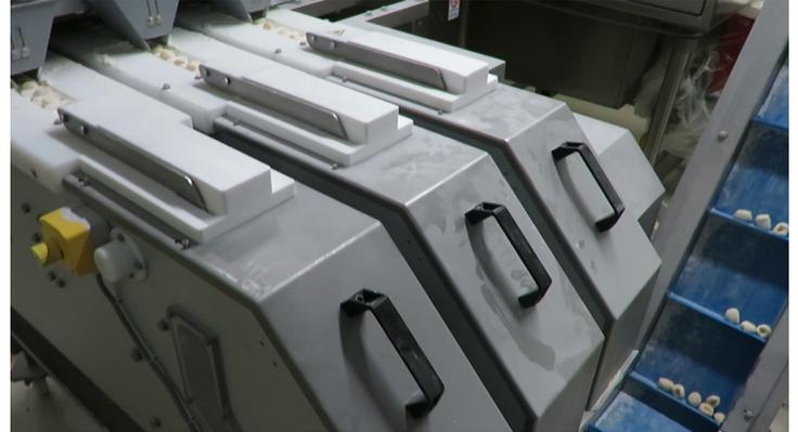
The Dumplings making machine (SGA) has been designed to make the “grandmother’s gnocchi”, pressed on the grater and embossed to hold sauces. The SGA machine extrudes the “gnocco” from the dough of potatoes and gives it the typical shape. The machine is composed by modular elements, one through four, according to the required productivity. The structure is made of stainless steel or plastic materials in compliance with food safety standards.
